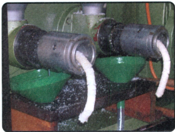
Plate 7. Dry processed virgin coconut oil extraction
